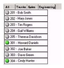
This area of the screen has a button defined for every extension that the user is monitoring. The attendant can define Extension Groups that include a specific set of extensions. The tabs at the top of the BLF Panel represent all of the defined Extension Groups. Selecting a different tab allows the attendant to view only the extensions that are included in that group.
