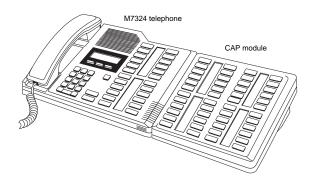
A CAP module is an add-on device that provides 48 extra memory or line buttons. You can connect one Norstar CAP module to the telephone to increase the number of lines it can handle.
