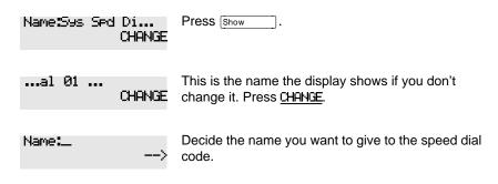
Press the telephone's numeric dial pad button that has the first letter of the name until the display shows the letter you want.
