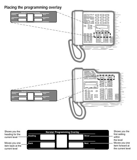
Programming buttons are active or inactive at different stages of programming. A button is active (meaning you can use that option), when the indicator next to it is lit ( $\triangleleft$  or  $\triangleright$ ).
