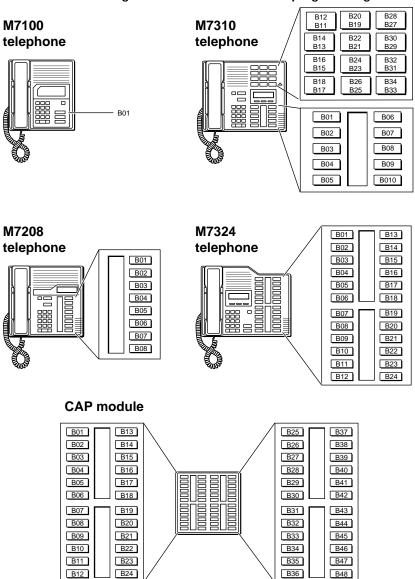
Use the display buttons to change the programming for a button. User Preferences programming cannot change the buttons that are used by lines, intercom, and the handsfree feature.
