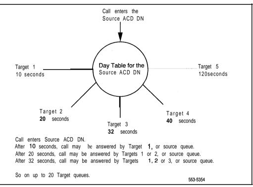
When a call is directed to the source ACD DN, the timer begins. The call rings until the first timer expires. After the timer expires, the calls can be answered by agents in Target 1. The system continues to track the wait time. When the timer for the second target expires, it is automatically included in the search. The call can now be answered by agents in the first target queue, or the second target queue. Targets continue to be added to the search as the timers expire.
