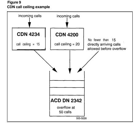
The CDN is covered by the Original Called Information category. The displaying of the CDN conforms to the current X11 software operation. Therefore, if a call initially dials a CDN, when that call is presented to or answered by an agent (depending on the agent's display class of service), the original called number, the CDN, is displayed.
