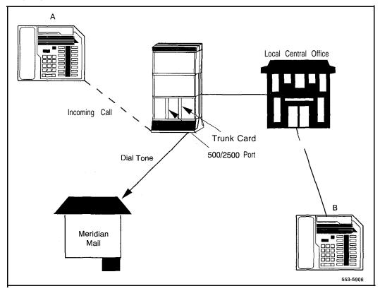
This illustration shows an outgoing call to from the Meridian 1 system to the Central Office. Station A transfers Station B to Meridian Mail and goes on-hook. The dialtone is provided by the 500/2500 type port with the new CLS LDTA after Station B disconnects.
