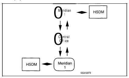
You can install a T1 link to different vendors and use the Meridian Communications Adapter (MCA) or QMT21 high speed data module to initiate or receive a 56 kb digital data call. The digital data call then transports across the vendor's digital network to another Meridian 1 or an SL-100.
