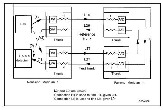
From Table 1 we can see that both pads will be switched IN at the far end. Therefore, the loss through the far end connection is  $1 \, dB \, (2 \, dB \, \text{in})$  the A to D direction and -1 dB in the D to A direction). The pad loss at the near end is the result of the  $2 \, dB \, \text{loss}$  in the A to D direction and the  $1 \, dB \, \text{gain}$  (such as -1 dB) in the D to A direction.
