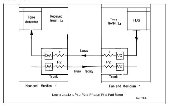
Figure 4 Near-end to far-end loss
