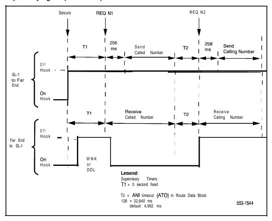
Figure 2 Supervisory signals (NT400/500 method)
