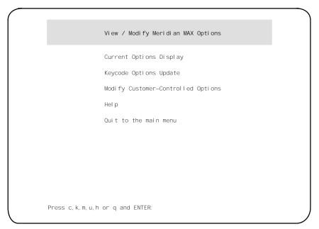
To access the View/Modify Meridian MAX Options submenu, shown in Figure 3-2, press v, followed by {**RETURN**}, from the main menu. This allows you to view the current options, modify customer-controlled options, and view the options on an application tape, as well as update the options from an application tape.
