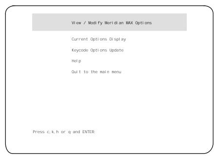
To access the View/Modify Meridian MAX Options submenu shown in Figure 2-2, press v, followed by {**RETURN**}, from the main menu. This selection allows you to view the current options as well as to update certain options using a keycode.
