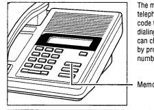
The memory button can store a telephone number or feature code to give you one touch dialing or feature activation. You can change the memory button by programming it with a new number or feature code.
