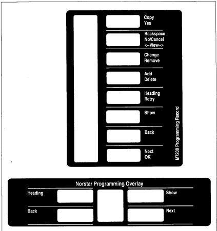
Programming Overlay for the M7208 Telephone (top) and for the M7310 and M7324 Telephones (bottom)
