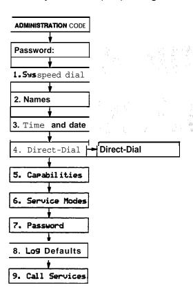
Use the **Show** button, the **CHANGE** display button and the dial pad to enter the internal number of the telephone to be designated as the Direct-Dial telephone.
