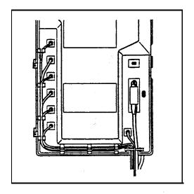
Figure 4 — Plugging in the 25-pair cable
