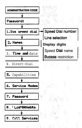
You can program 70 System Speed Dial codes ranging from #01 to #70.
