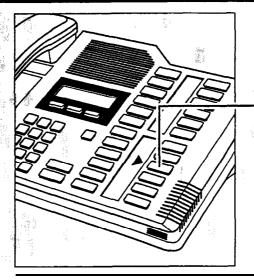
Memory buttons are the buttons with indicators other than line or Handsfree buttons. Memory buttons store telephone numbers or feature codes to give you one touch dialing or feature activation. You can change what a memory button does by just programming it with a new number or feature.
