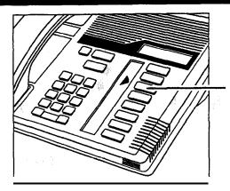
Memory buttons are the buttons with indicators other than line or Handsfree buttons. Memory buttons store telephone numbers or feature codes to give you one touch dialing or feature activation. You can change what a memory button does by just programming it with a new number or feature. You cannot program a line or Handsfree button.
