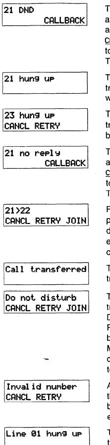
The person to whom you transferred an external call has Do Not Disturb active on their telephone. Press <u>CALLBACK</u> or the flashing line button to reconnect to the call. On the M7100 Telephone, lift the receiver.
