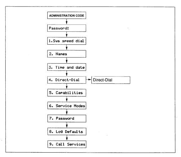
Use the <u>Show</u> button, the <u>CHANGE</u> display button and the dial pad to enter the internal number of the telephone to be designated as the Direct-Dial telephone.
