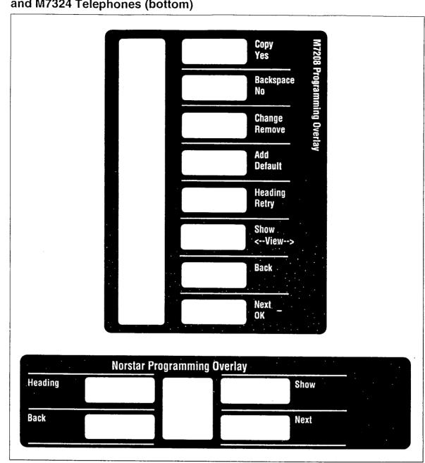
Programming Overlay for the M7208 Telephone (top) and for the M7310 and M7324 Telephones (bottom)
