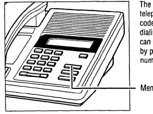
The memory button can store a telephone number or feature code to give you one touch dialing or feature activation. You can change the memory button by programming it with a new number or feature code.
