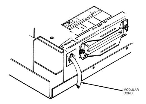
**Note 1:** Connect modular cord to the LC13 circuit pack through the appropriate connecting block.
