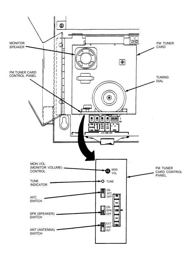
Figure 2-10. FM Tuner Card Controls and Indicator
