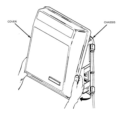
Figure 2-1. Removing PagePac VS Cover
