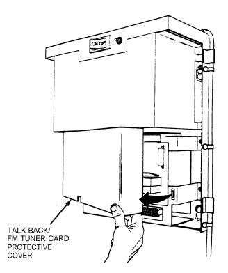
Figure 2-3. Opening PagePac VS Talk-Back/FM Tuner Card Protective Cover
