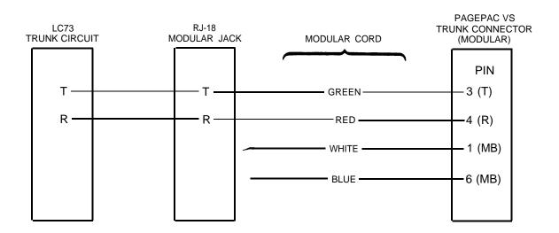
Note 2: The LC73 uses only the tip and ring, or pins 3 and 4 as indicated. Pins 2 and 5 are not used at all. Pins 1 and 6 provide a busy out feature not used with the HORIZON CS.
