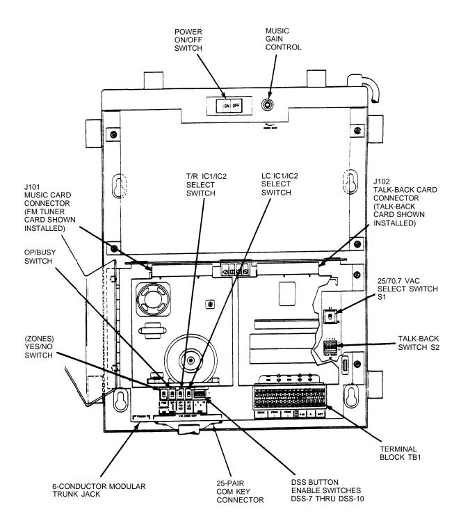
Figure 1-2. PagePac VS Connectors, Switches, and Controls (Cover Removed)
