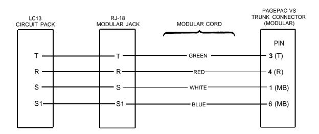
Note 2: Only half of the LC13 circuit pack is required when connecting to the Page Pac VS. The S and S1 connections are required only when MAKE BUSY function is provided (see OP/BUSY switch. Table 1-B).
