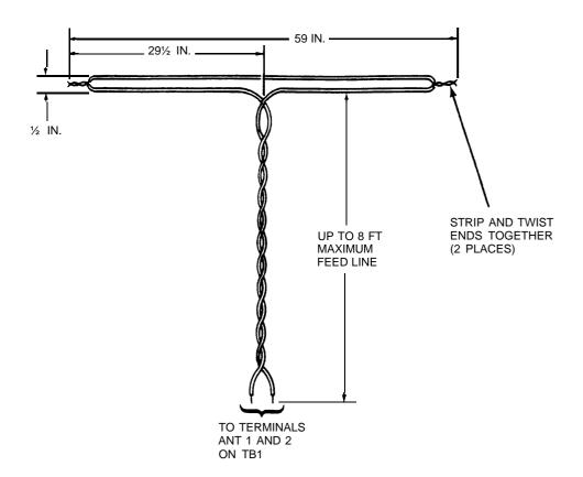
Note 1: Make from 22 AWG twisted-pair wire or TV twin lead.
