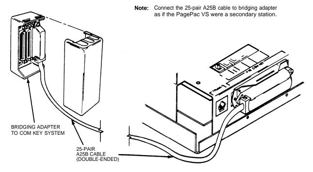
Figure 2-7. Cable Connections to Com Key System
