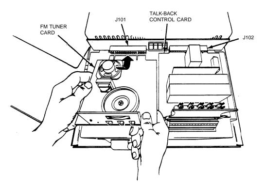
Figure 2-4. Installation of Optional Circuit Cards
