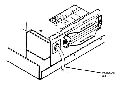
**Note 1:** Connect modular cord to the LC73 trunk circuit through the appropriate connecting block.
