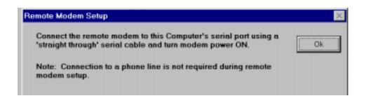
4. Complete the instructions on the screen and click **OK**. The next screen to be displayed requests selection of a COM Port. Select the proper COM Port and click **OK**.
