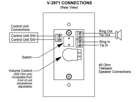
**NOTE:** When utilizing the V-2971 volume control with 45 Ohm talkback speakers featuring an integrated volume control or volume preset capability, set the volume at the speaker to maximum. This will allow full volume range from the V-2971 volume control.
