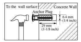
**3.** Install the screws (included) into the anchor plugs.
