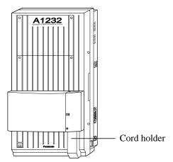
**10.** Fix the cords to the wall as shown so that the front cover can be opened.
