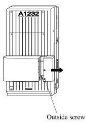
**5.** Secure the inside screw (included) to fix the cabinet to the main unit.
