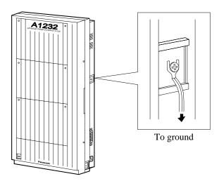
In most of the continental United States, the ground provided by the "Third wire ground" at the commercial power outlet will be satisfactory. However, in a small percentage of cases this ground may be installed incorrectly. Therefore, the following test procedure should be performed.
