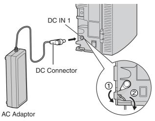
3. Plug the AC cord into the AC adaptor, and then plug the other end into an AC outlet.
