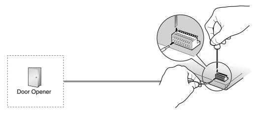
2. Attach the terminal blocks to the connectors of the DPH4 card in the PBX.
