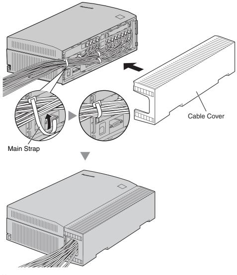
5. Bind all the connected cables together using the main strap, and then close the cable cover. For how to close the cable cover, refer to "2.2.3 Opening/Closing the Covers".
