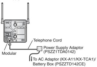
**4.** Install the CS temporarily for the site survey. Install the CS at least 2 m (6.6 ft) above the floor, keeping the antennas in the upright position.
