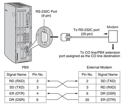
After connecting the PBX and the external modem, set the power switch of the external modem to "ON", then the external modem will be initialized with the default values.
