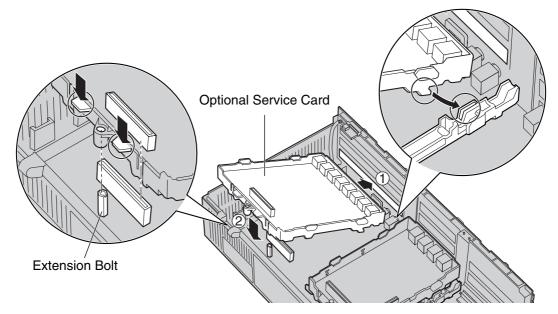
**3.** Insert the new extension bolt (included with the card) into the hole on the card, and tighten it to secure the card.
