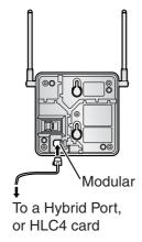
**2.** Pass the cable through the groove of the CS (in any direction depending on your preference).
