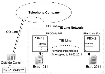
An outside caller dials "123-4567". The call reaches the destination (extension 1011 of PBX-1), and the call is forwarded, transferred, or intercepted to extension "2011" of PBX-2 through the TIE line.
