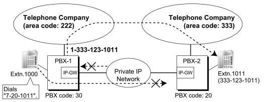
The leading numbers of extensions accessed through the VoIP network are added as entries to the Quick Dialing table, in addition to being registered as Other PBX Extension Numbers, as shown below: **[Programming Example]**
