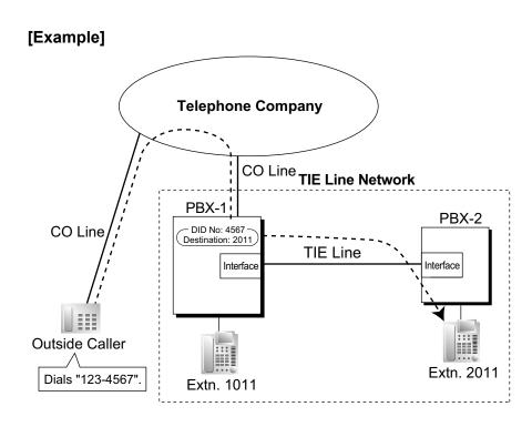
An outside caller dials "123-4567". The call is sent to extension "2011" of PBX-2 through the TIE line according to the assignment of the DID or DIL call destination of PBX-1. ( $\rightarrow$  4.1.5 DID (Direct Inward Dialing))
