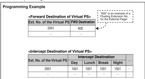
When extension 2001 is called from another extension or is the first destination of an incoming CO line call, etc., the call will ring at extension 600 (external pager) first, and then ring at the intercept destination (extension 1001) after the IRNA Timer expires.
