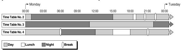
Note that time modes can be arranged as they are needed (for example, night mode can occur in the morning and afternoon, if necessary) and not all time modes need to be used in a tenant's time schedule.
