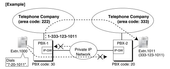
The leading numbers of extensions accessed through the VoIP network are added as entries to the Quick Dialing table, in addition to being registered as Other PBX Extension Numbers, as shown below:
