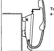
To temporarily set the handset down during a conversation, place it as shown here.
