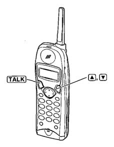
Lift the handset off the base unit and press ▼ or ▲ to enter the Caller List.
