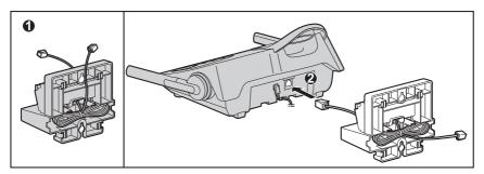
3 Insert the hooks on the wall mounting adaptor into the holes (A) and (B) on the base unit.
