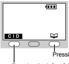
Three soft keys are used to select functions displayed directly above each key. Functions displayed above each key will change depending on the state of use.
