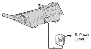
2 Tuck the telephone line cord inside the wall mounting adaptor (1).Connect the telephone line cord (2).
