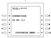
2. The 3101 setting screen appears. Enter the 4-digit ID number and press **HOLD** key to make setting. Each time the **HOLD** key is pressed, the setting changes:
