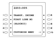
4. Enter the first CO (Exchange) line or private line number using the 10-key pad. (The figure on left shows setting of block No. 03.)
