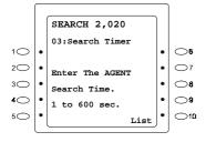
3. Set parameter 2, and press the **HOLD** key. Example: Press keys **0**, **1** and **5** to set the Search Timer to 15.
