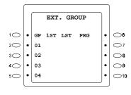
3. The following screen appears. Press the **soft** key for desired block number.
