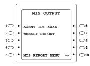
5. Once the input data is validated, the data output starts. The following screen appears while the output is in progress. To abort output, see the section [MIS data output abort], section, [Other Features]
