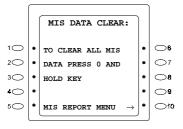
3. The following screen appears. To clear data, press **0** and **HOLD** keys. This starts data clear processing.
