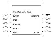
1. Press the **soft** keys (**1** to **6**) for the commands to be set, and press the **HOLD** key.
