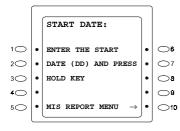
5. The following screen appears. Enter the starting date and ending date of the data to be output. First enter the starting date, press **HOLD** key to validate, then enter the ending date and press **HOLD** key again. No month is needed to be entered. For example, data for a period beginning with April 25 and ending with May 2, Enter 25 as the starting date, 2 as the ending date. For 1 through 9, 01 through 09 can be entered instead.
