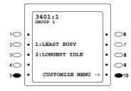
3. First setting (3401) for the selected group is displayed. Enter a set value, then press the **HOLD** key to validate setting. Every time the **HOLD** key is pressed without set values specified, the next setting item is displayed. Press **FL/R** key to return to the previous setting.
