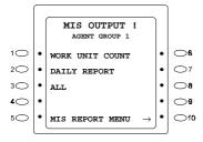
5. Once the input data is validated, the data output starts. The following screen appears while the output is in progress. To abort output, see the section [MIS data output abort] section, [Other Features].
