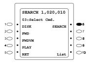
1. Press **soft** keys (**1** to **6**) for the command to be set, and press the **HOLD** key.
