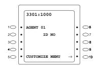
4. Enter 4-digit ID number using the 10-key pad. (The figure on left shows setting of Agent No.01.)
