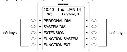
You can easily access and use many telephone features by pressing the soft key next to the desired Main Menu item. These items include:
