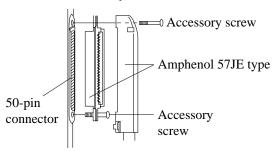
**2.** To attach the Amphenol 57JE type (Plug) to the connector, drive the accessory screw into the upper part.
