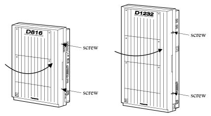
**3.** Tie together all of the connected cords and attach them to the wall so that the cords cannot be pulled out of the main unit.
