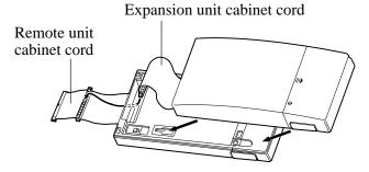
**3.** Remove the cover plate and connect the cabinet cord to the connector in the main unit firmly.
