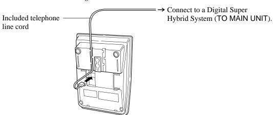
KX-T7440 and KX-T7441 can be connected to a KX-T7400 series digital proprietary telephone.
