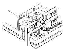
2. Replace the cover and tighten the screw.
