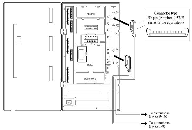
3. After inserting the connector, fasten the connector with the nylon tie.
