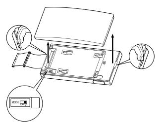
**2.** Attach the expansion unit to the Remote Unit as shown below. Be sure to connect the cabinet cords by inserting the expansion unit cabinet cord through the slot in the Remote Unit.
