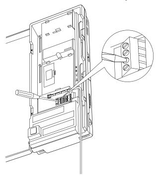
**3.** Insert the wires coming from the door openers into holes and tighten the screws. Pass all the wires through the Holder.
