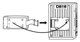
**3.** Hook the cabinet onto the main unit and slide the cabinet to the left until it is secured.
