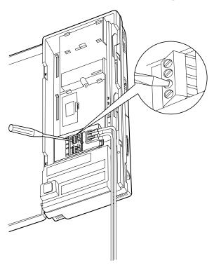
**3.** Insert the wires coming from the door openers into holes and tighten the screws. Pass all the wires through the Holder.
