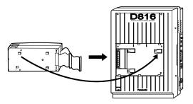
**4.** Hook the cabinets onto the main unit and slide the cabinets to the left until they are secured.
