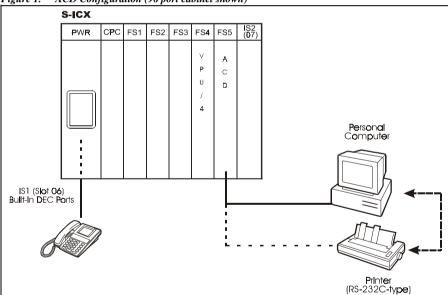
Figure 1. ACD Configuration (96 port cabinet shown)
