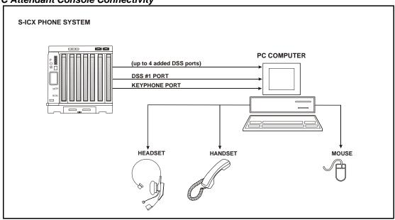
This product is offered in two capacities: a **2-port solution** (equivalent to one 24-key phone with one DSS/72 console) which is capable of monitoring up to 96 ports; and a **6-port solution** (equivalent to one 24-key phone with four DSS/72 consoles) which supports a maximum of 384 ports.
