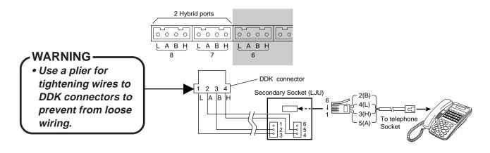
NOTE: In this manual "T" and "R" on the PCB have been replaced with "A" and "B", respectively, in the description.
