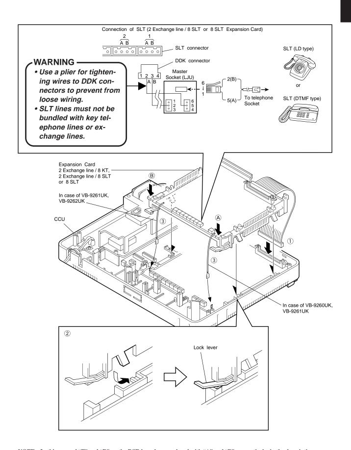
NOTE: In this manual "T" and "R" on the PCB have been replaced with "A" and "B", respectively, in the description.
