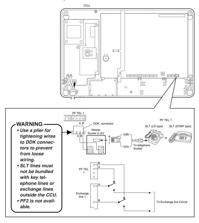
NOTE: In this manual "T" and "R" on the PCB have been replaced with "A" and "B", respectively, in the description.
