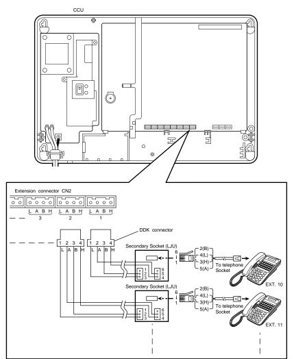
NOTE: In this manual "T" and "R" on the PCB have been replaced with "A" and "B", respectively, in the description.
