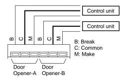
NOTE :  $\bullet$  Terminals C and M are used for Make controlled devices.
