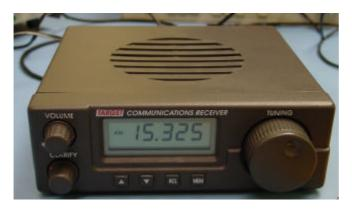
**Summary.** The receiver was modified and capable of receiving DRM, but performance was limited by the phase noise from the 1<sup>st</sup> Local Oscillator (LO).
