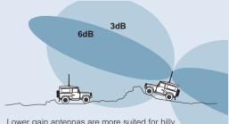
Lower gain antennas are more suited for hilly terrain where reception does not depend on the angle of the antenna.
