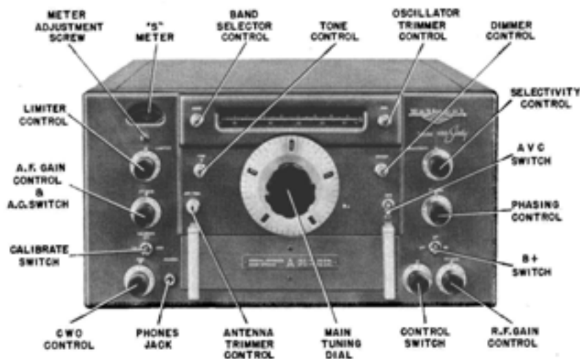
Figure No. 5. Front View of Receiver
