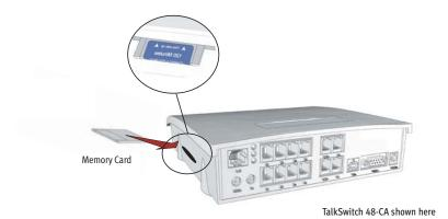
Make sure the gold contact is face down and inserted into the MEMORY SLOT first. The "This side up" tab should be showing.
