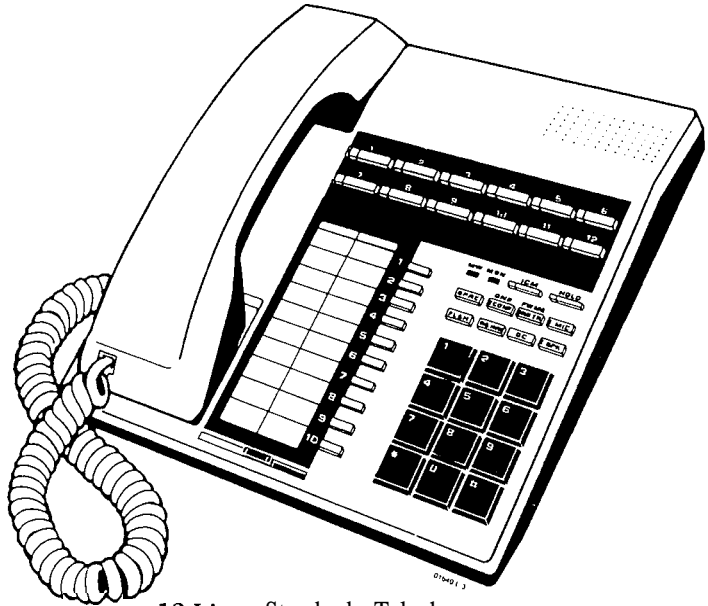
12-Line Standard Telephone
