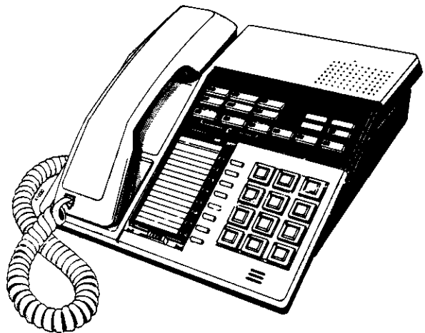
Figure 2-1 KEY TELEPHONE, EK-616, KEY DESIGNATIONS
