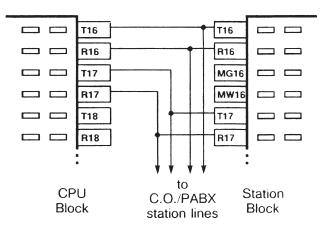
Connect T (Tip) and R (Ring) from each monitored station to the associated T and Rpins on CPU block #2. The 524 is connected in parallel with the station lines.
