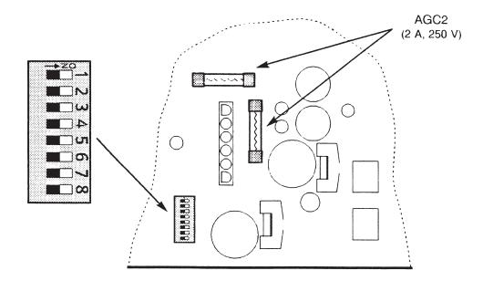
Figure 8 – CPU Option Switches and Fuses
