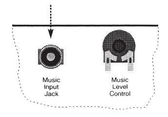
1. Connect an RCA-type phono plug to one end of a single conductor shielded cable, or obtain a cable with a plug attached. The center conductor connects to the pin of the plug.
