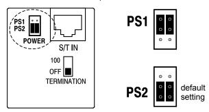
Using an 8-conductor line cord, connect the S/T IN jack on the telephone to the TERMINAL jack on the NT1. Route the cord under the guide tabs in the phone base.
