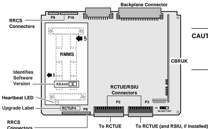
**CAUTION!** When removing the RMMS from RCTUF, take off the RMMS slowly, rocking back and forth in the direction of the arrows in the diagram.
