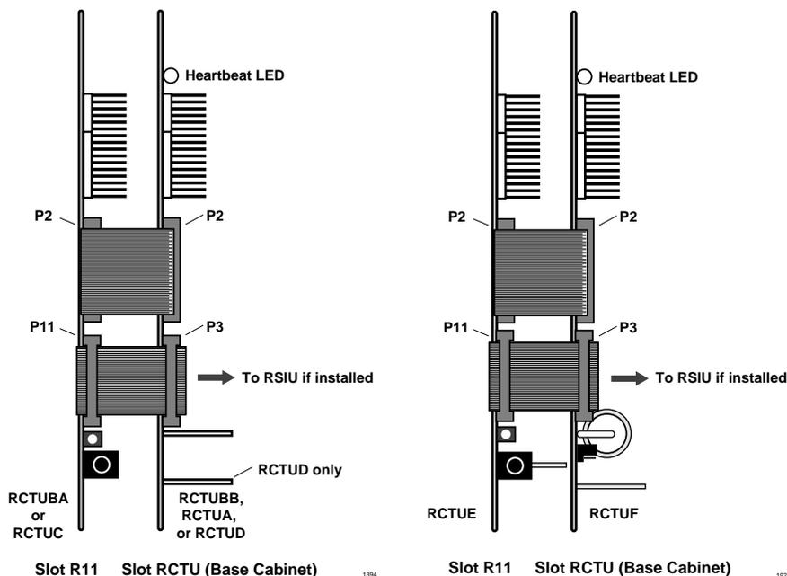
**Figure 1 RRCU PCB Removal and Component Placement**
