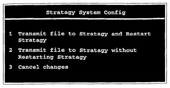
Press 1; the changes are transmitted to Stratagy and Stratagy is shut down and restarted. **By** shutting down and restarting Stratagy, the changes take effect.
