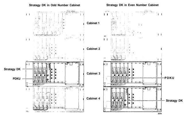
Figure 3 Stratagy DK424/DK280 PDKU DSS/Busy Lamp Field Slot Assignment Examples (console-slot-id configured as 0)
