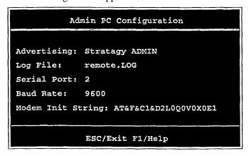
**Note** Press F2 in the Serial Port and Baud Rate fields to display a pop-up box with valid entries.
