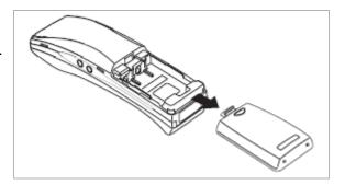
Connect the battery pack connector, observing correct polarity to the jack inside the battery compartment, as shown on the right.
