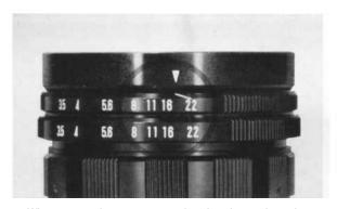
When a manual pre-set aperture lens is to be used, set the pre-set aperture ring to the reading of the smallest aperture, before the ring is turned to secure a correct exposure.
