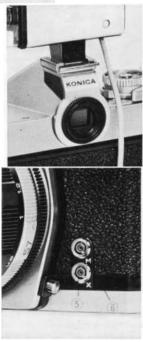
For synchroflash photography, use the Accessory Clip III on which either a synchroflash gun or a small electronic light unit may be mounted. As your camera is equipped with a tap-hole each for Classes M and X, insert the plug into the Synchroflash Contact Tap-hole "M" .6' for bulbs of Classes M and FP or the Synchroflash Contact Tap-Hole "X" 5) for electronic lights and bulbs of Class F. This manual was created by www.butkus.org/chinon and should only be found at my site.
