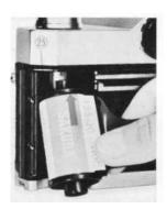
$2\ {\hbox{Direct toward the underside of the camera that side of the cartridge through which its spindle sticks out and put the cartridge into the Cartridge Chamber $2$ .}$
