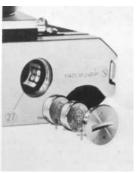
The compound CdS meter of the KONICA AUTOREFLEX A takes two 1.3V mercury battery cells as its electric source. Wipe the mercury battery cells, accessories for camera, with a piece of dry and clean cloth and put them into the mercury battery chamber.
