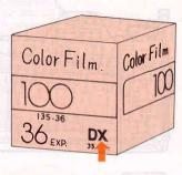
This camera automatically sets the ISO film speed of DX-coded film when it is loaded into the film chamber. Therefore, you are recommended to use only DX-coded film in this camera. (If non-DX film is loaded the camera will automatically set the film speed to 100, whatever film speed it may have; in other words, the only non-DX film usable for this camera is one with ISO 100.)
