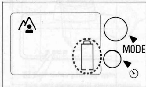
Slide the main switch to "ON". Replace the battery when the symbol is indicated as illustrated.
