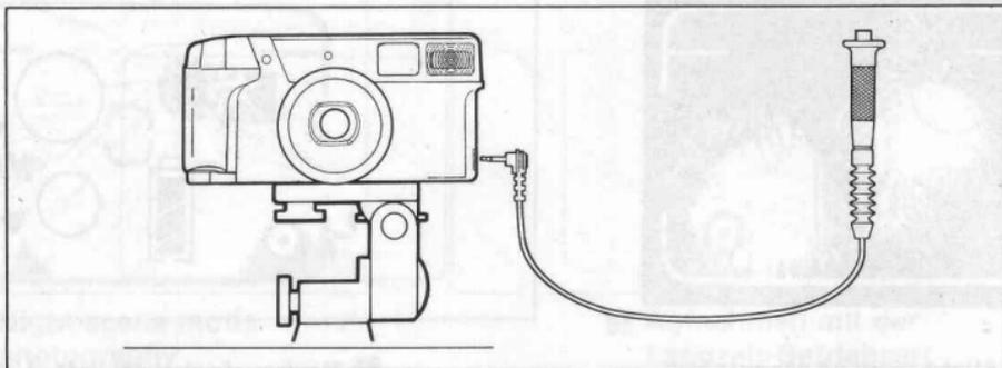
If there is a risk of camera shake, it is best to use a tripod and an electromagnetic release (these are not included).
