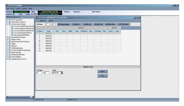
3.) CO Line ISDN Attributes (PGM 143) – Set the COLP and CLIP Table Idx fields to 0, set the Call Type to Subscriber, the DID Conv Type to 2 (for integration with Flexible DID Table, PGM 231), set the DID Remove Num to 7 (or other entry if the carrier is sending more than 10 digits), and turn ISDN ENBLK Send to On.
