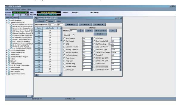
2.) **CO Line List (PGM 140)** – If the SIP carrier will be providing DID (direct inward dialing) trunks, program the VoIB trunks used for SIP integration as ISDN DID.
