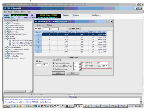
7.) VolB/Gatekeeper Setting (PGM 340) – Program the IP Address, Gateway Address, Subnet Mask for the VolB card. Set the VolB mode to SIP unless the system is networked with another system, if so, use the DUAL option. Program the DTMF Mode so it matches the same field in PGM 322.
