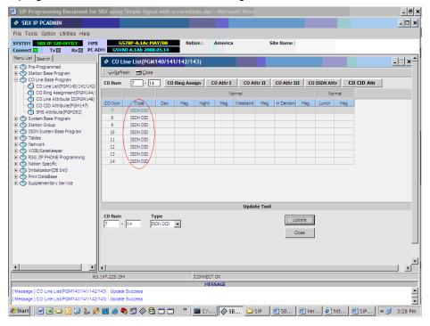
3.) CO Line ISDN Attributes (PGM 143) – Set the COLP and CLIP Table ldx fields to 0, set the Call Type to Subscriber, the DID Conv Type to 2 (for integration with Flexible DID Table, PGM 231), set the DID Remove Num to 7 (or other entry if the carrier is sending more than 10 digits), and turn ISDN ENBLK Send to On.
