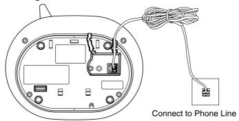
Plug one end of the telephone line cord into the jack on the bottom of the base unit. Plug the other end of this cord into the wall jack.
