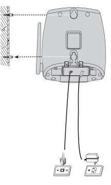
4. Connect the power cord. Plug the DC connector into the DC jack at the rear of the base unit. Plug the AC power adapter into an electrical outlet.
