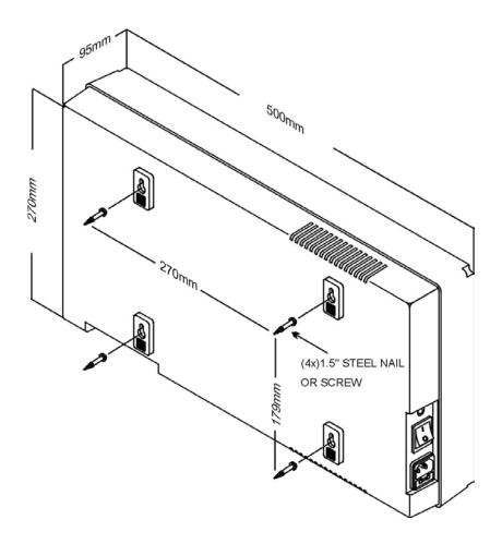
Figure 6: HOW TO WALL MOUNTING
