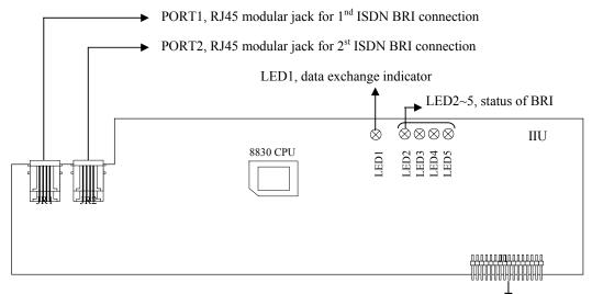
J1, 16 x 2 pin male connector, connect to J3 or J4 on motherboard
