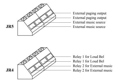
Figure 2 : Optional Equipment terminal PIN Functions
