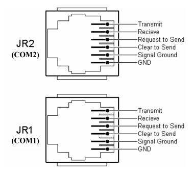
Figure 3 : Serial Port Jack Pin Functions
