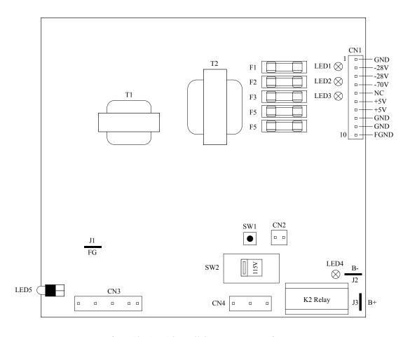
Figure 19: ATLAS EX 60 System power supply
