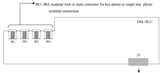
J1, 16 x 2 pin male connector, connect to J4/J6/J8/J9 on motherboard
