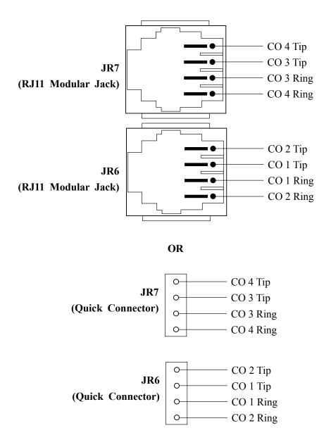
Figure 7: Typical Trunk Connecting Jack Pin Functions
