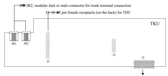
J1, 16 x 2 pin male connector, connect to J2 or J4 on motherboard
