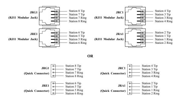
Figure 9: Typical Station Connecting Jack Pin Functions
