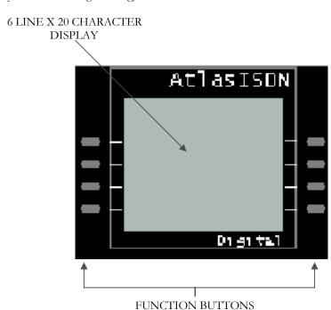
Each line of the display can have up to 20 characters. The bottom four lines of the LCD display are used to show functions that are available to you. To select a function simply press the button next to that function. When a button is pressed, the
