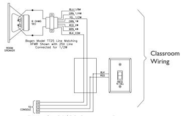
Figure 1 - CA15C Connecting Diagram
