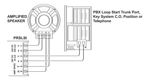
**Note:** The AMP SPKR "T" and "R" outputs are balanced and should not be connected to Ground.
