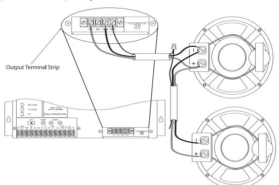
Figure 7: Speaker Connection, Output Wiring
