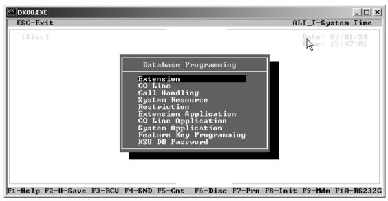
While you are programming the database using PC-DBA programming, the system stores any changes you make in its working directory—not in the DX-80 system memory. When you have finished making your programming changes, you must perform a SEND operation. They system then overwrites the system memory with whatever you have programmed into the working directory. Until you perform the SEND command, **none of your changes are in effect**.
