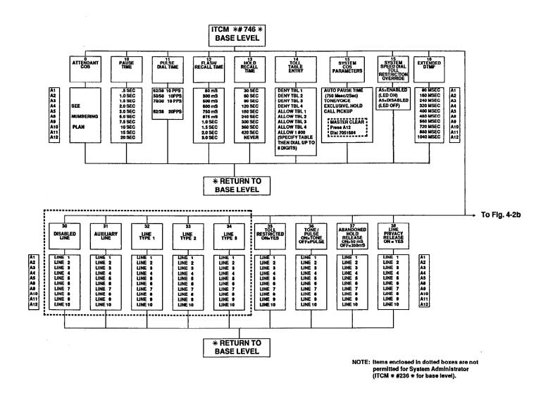
Figure 4-2a. System Programming Block Diagram
