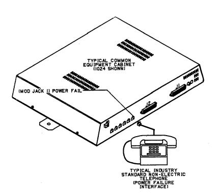
Figure 3-5. Power Failure Station Connection.
