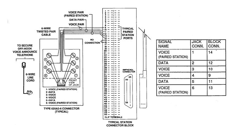
Figure 3-4 Secure Off-Hook Voice Announce Connections
