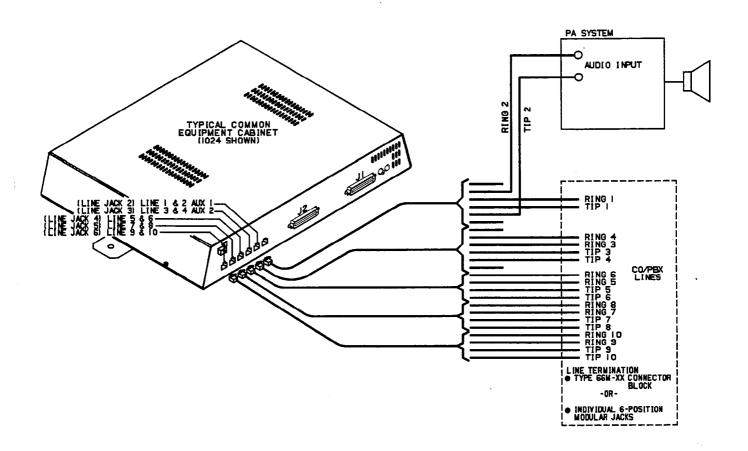
Figure 3-8. External Paging Interface - Line Port
