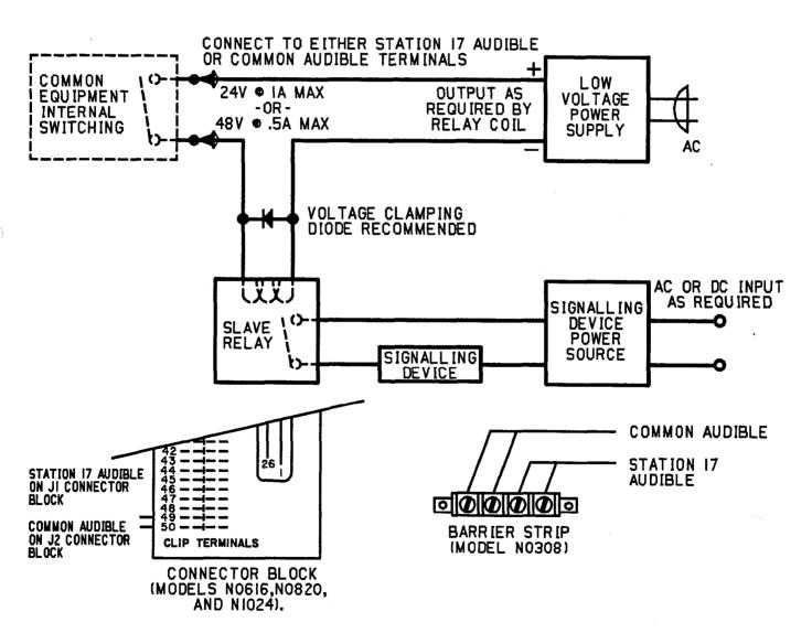
Figure 3-6. Common Audible and Auxiliary Station Interface
