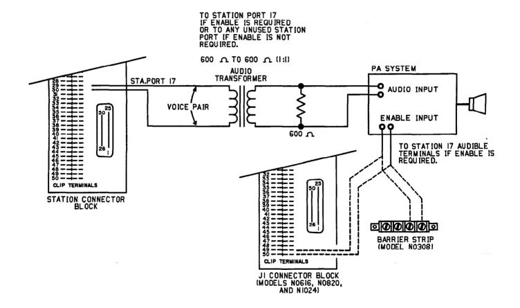
Figure 3-7. External Paging Interface - Station PA Port
