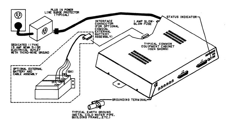
Figure 3-2. AC Power Connection and System Grounding
