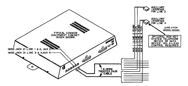
Figure 3-9. Auxiliary Equipment Interface Connections
